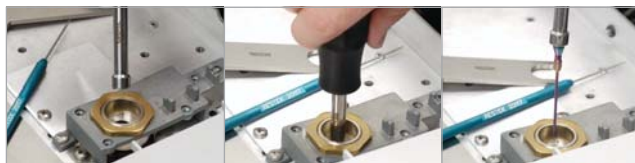
Slip tool over FID jet... ...loosen jet... ...and remove.
