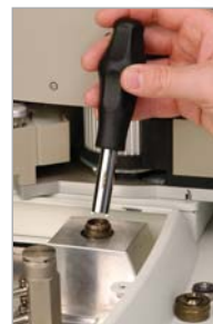
Remove septum cap, septum holder, septum, and septum support.
