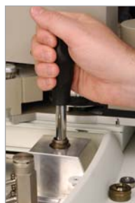
Turn counter-clockwise to loosen liner cap.
