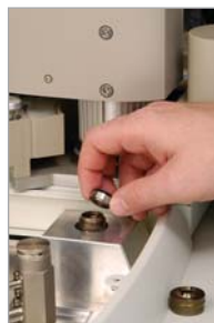
Remove septum cap, septum holder, septum, and septum support.
