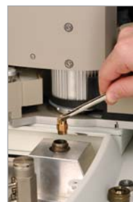
Use tweezers (cat. #20101) to remove liner cap.
