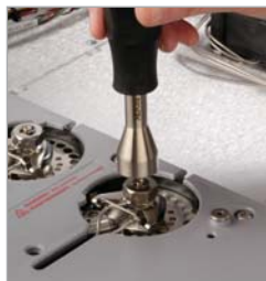
Slip tool over septum nut...
