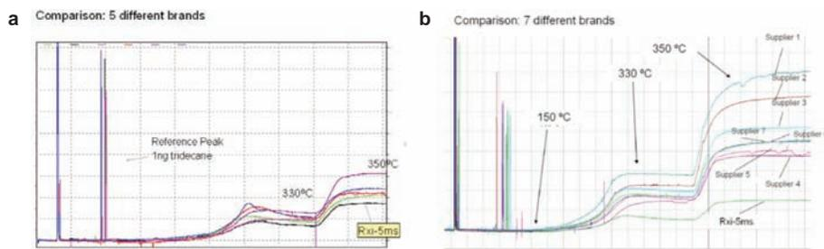
*Figure 2* Bleed comparison of different types of 5% diphenyl and aryl phases: a) 0.25- $\mu\text{m}$  film, b) 0.5- $\mu\text{m}$  film.
