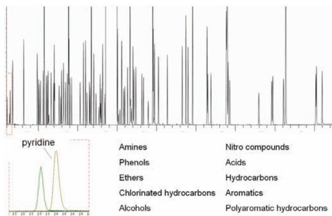
Figure 10 A multicomponent environmental analysis such as U.S. EPA 8270 is usually analyzed using an Rxi-5Sil MS column. All groups of compounds elute as symmetrical peaks. (See Table 3 for conditions.)
