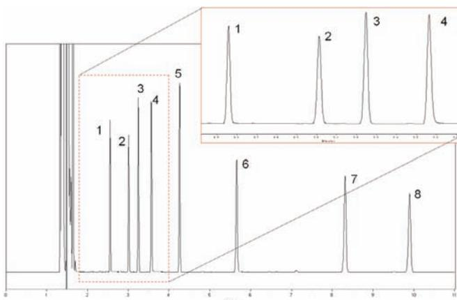
Figure 9 Standard test of Rxi-5Sil MS columns. Column: 30 m × 0.25 mm,  $df = 0.25 \mu\text{m}$ . 1) 2,6-hexanediol, 2) 4-chlorophenol, 3) methylnonanoate, 4) 1-decylamine, 5) tridecane, 6) undecanol, 7) acenaphthylene, 8) pentadecane.
