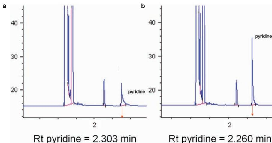
*Figure 4* Impact of column activity on retention of pyridine peak. a) State-of-the-art column deactivation, b) Rxi column deactivation.
