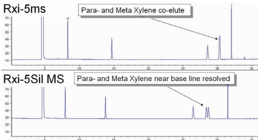
Figure 8 Separation of xylenes on Rxi-5ms and Rxi-5Sil MS columns, both 60 m × 0.25 mm,  $df = 0.25 \mu\text{m}$ , temperature = 35 °C.
