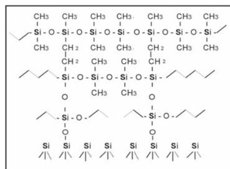
Figure 1 Schematic representation of Rxi bonding process (cross-bonding, surface bonding, deactivation, and shielding for minimization of impact of [re]active silanols).
