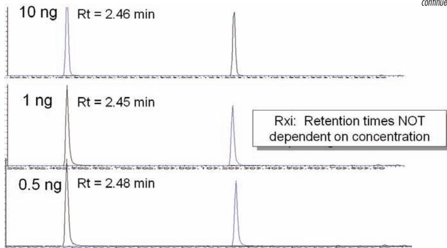
Figure 7 Peak shape and retention of 10, 1, and 0.5 ng pyridine on similar column dimensions as in Figure 8, using Rxi column technology.
