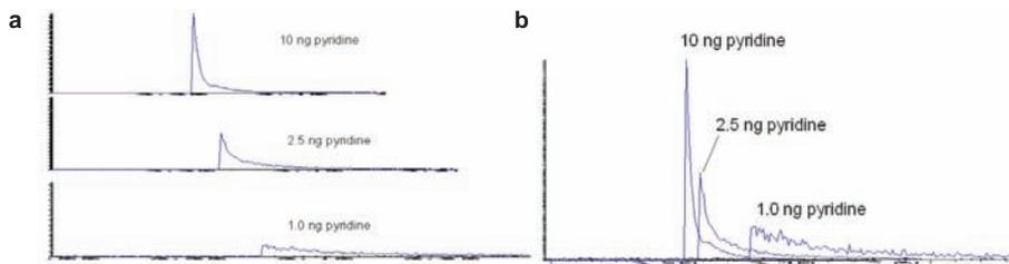
Figure 6 Impact of the amount of active compound injected on retention time and peak shape. Peak shown: pyridine at 10, 2.5, and 1 ng on a conventional state-of-the-art column ( $30\text{ m} \times 0.25\text{ mm}$ ,  $df = 0.25\text{ }\mu\text{m}$ ). a) Individual runs, b) overlaid chromatograms.
