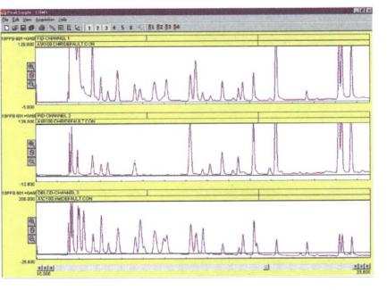
These three chromatograms are from an analysis of Method 8021 standard plus gases on an SRI Environmental GC system. Peak identities can be confirmed by comparing the results from the three different detectors. Peaks which often coelute, such as benzene and carbon tetrachloride, can still be measured since the PID responds only to the benzene, while the DELCD only responds to the carbon tetrachloride.
