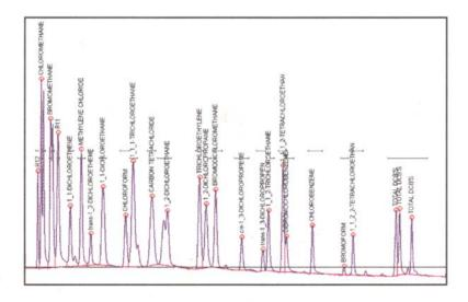
The DELCD chromatogram is shown at left in more detail and with the peaks labeled for identification. The DELCD is completely selective for compounds containing chlorine and/or bromine. Other analytes do not respond at all, even at very high levels. The DELCD actually operates on the FID's exhaust gases; therefore, all contaminants are precombusted by the FID to CO<sub>2</sub> and H<sub>2</sub>O.
