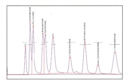
The first few peaks in the 8021 standard, including vinyl chloride, are of special interest to many analysts. The chromatogram to the left shows the expanded detail of the first few peaks in the analysis (the VOC gases). Note the exceptionally good resolution and peak shape delivered by the SRI system with its dual trap technology.
