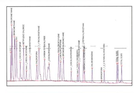
The first few peaks in the TO-14 standard, especially vinyl chloride, are of special interest to many analysts. This chromatogram shows the expanded detail of the first few peaks (the VOC gases) in the analysis shown above. Note the exceptionally good resolution and peak shape delivered by the SRI system's dual trap technology.
