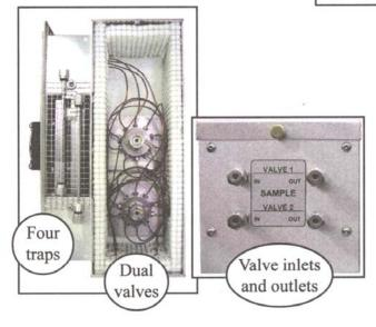
This SRI GC has been customized with a dual TO-14 Air Concentrator: four traps, and two gas sampling valves.
