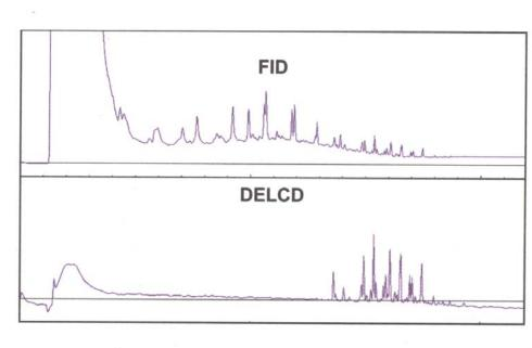
The PCB GC System is also useful for detecting pesticides, PAHs, JP-4, kerosene, and diesel in soil. Soil samples are typically 20-50% water, so the FID flame is automatically relit after a large water peak. The 30 meter capillary column is included to efficiently separate hydrocarbons up to  $C_{40}$ +. The built-in, "whisper quiet" air compressor provides an infinite supply of combustion air for the FID detector, and if used with the  $H_2$ -50XR hydrogen generator, no cylinders are required.
