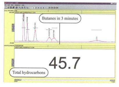
The PeakSimple data system controls the automated valve injection sequence and displays both the continuous total hydrocarbon reading as well as the separated peaks. An alarm function alerts the operator for any out-of-range readings. Summary reports are easily printed or copied to Excel or similar programs.
