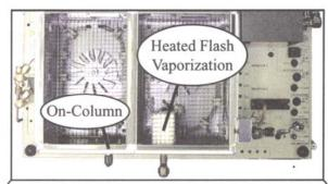
This 8610D GC has a standard On-Column Injector on the first oven, and an optional Heated Flash Vaporization Injector on the second oven.
