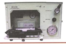
The handy storage compartment built into the front of the 210 holds your injection syringe, priming syringe, spare parts, and a few vials securely during shipping. Keep your HPLC tools with your HPLC.
