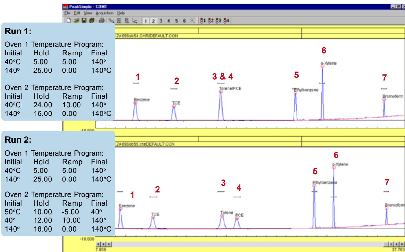
As seen in the Oven 2 temperature program for Run 2, PeakSimple provides negative programming capability in addition to unlimited ramping. Making this slight change in Oven 2's temperature program not only separated Toluene and PCE, it also altered the retention times of Ethylbenzene and o-Xylene. The TCS GC gives you the power to move peaks!
