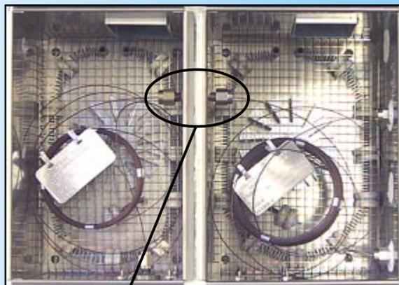
***In addition to the independent temperature control, a mid-point pressure control adds even further separation capability—for the serious chromatographer:***
