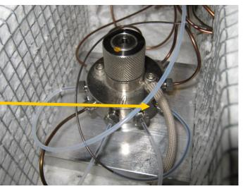
Sulfur analysis at the ppb level is difficult because sulfur sticks to many surfaces (adsorption). For this reason only Teflon or other extremely inert tubing can be used.
