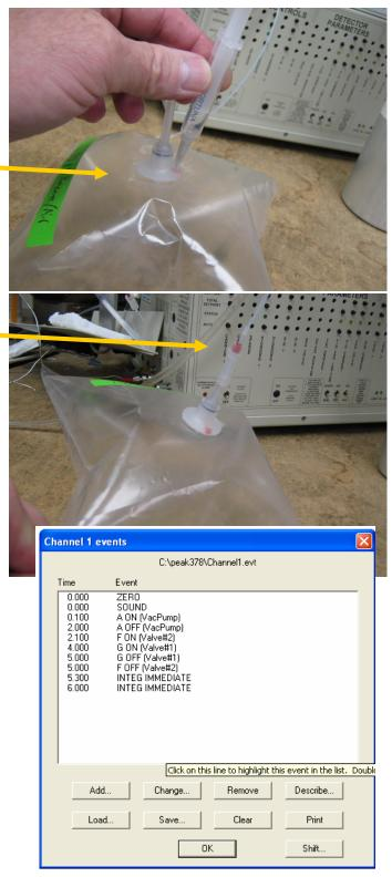
The event table has Relay A (the vacuum pump) turned on from .1 minutes to 2 minutes so the vacuum pump sucks the sample in the Tedlar bag through the trap for 1.9 minutes at the beginning of the analysis. The trap is at room temperature (25C).
