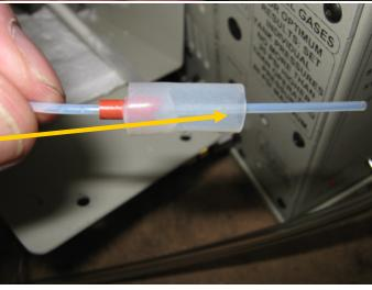
The trap which pre-concentrates the sulfur molecules is located between the ducts of the valve oven. Remove the cover by loosening the four brass thumbscrews.
