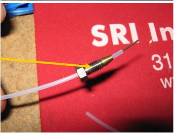
Teflon tubing must also be used to transport the sample into the GC from the Tedlar bag or other sample container. Note how the normal swagelok sample inlet fitting has been drilled out to allow the Teflon tubing to pass through.
