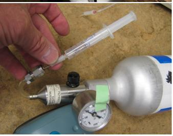
Inject the H2S standard mixture into the Tedlar bag through the septum in the bag. In this case we are injecting 1ml of 100ppm H2S into 1000ml (1 liter) of air in the bag. This results in a dilution of 1000 times so the resulting concentration of H2S in the bag is 100 ppb (parts per billion). Add any other sulfur molecules in the same way.
