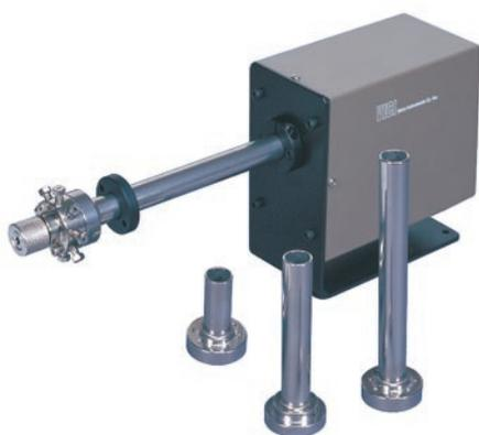
Valves which will be installed in ovens or heated zones require a standoff assembly, which locates the actuator out of the heated zone and supports both the valve and the handle or actuator. The 5/8" outside diameter standoff tube extends through the oven wall and is secured by means of a clamp ring supplied with the assembly.
