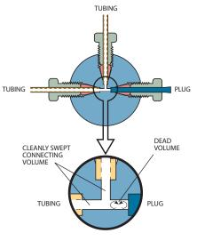
access points to "distribute" a gas or liquid through a system. *CAUTION!* Using a distribution fitting in reverse to coalesce multiple streams may create dead volume. Special manifolds are available for this application.
