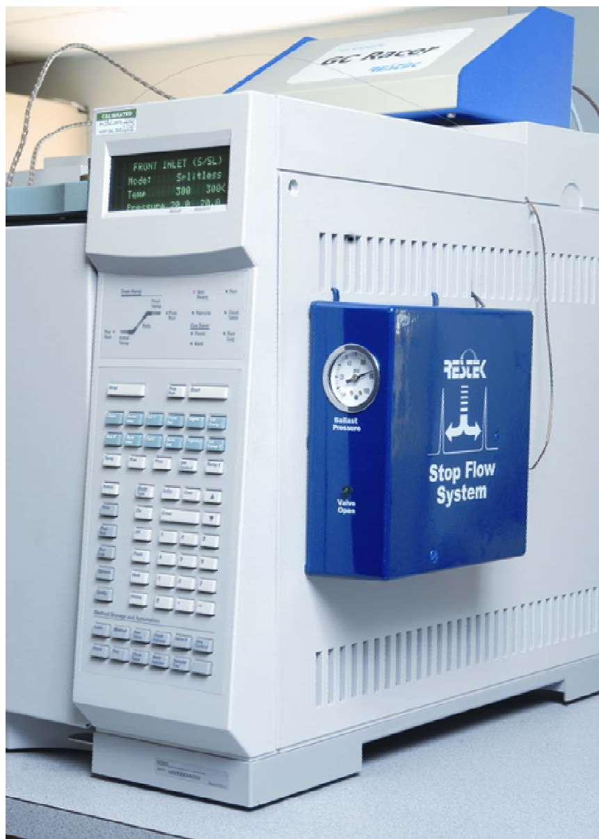
Figure 10. The stop-flow system connected to a gas chromatograph
