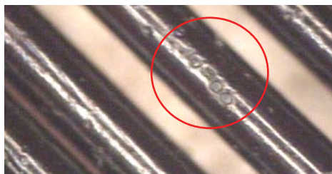
HT fused silica columns, labeled as stable to 430°C, show pitting and breakdown.
