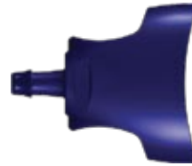
SBLF013-CM030 Side Latch Quick Connect Female 500 Series Barb 1/8" (3.2 mm) ID Tubing, Blue Nylon A: .935" B: 2.037" C: .467" Also available in Grey Nylon - SBLF013-8B
