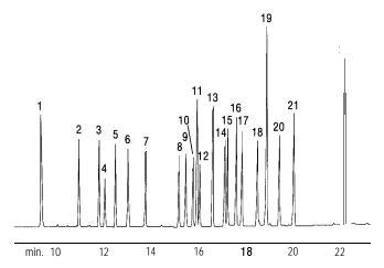
30m, 0.32mm ID, 0.50µmRtx-CLPesticides column (cat # 11139) run in parallel with the Rtx-CLPesticides2 column. Oven temp.: 120°C (hold 1 min.) to 300°C@ 9°C/min, (hold 10min.); Oead time: 1.4 min. Carrier gas: He.
