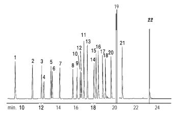
30m, 0.32mm ID, 0.25µm Rtx-CLPesticides2 column (cat # 11324) run in parallel with the Rtx-CLPesticides column. Oven temp.: 120°C (hold lmin.) to 300°C@ 9°C/min. (hold 10min.); Dead time: 1.4 min. Carrier gas: He.
